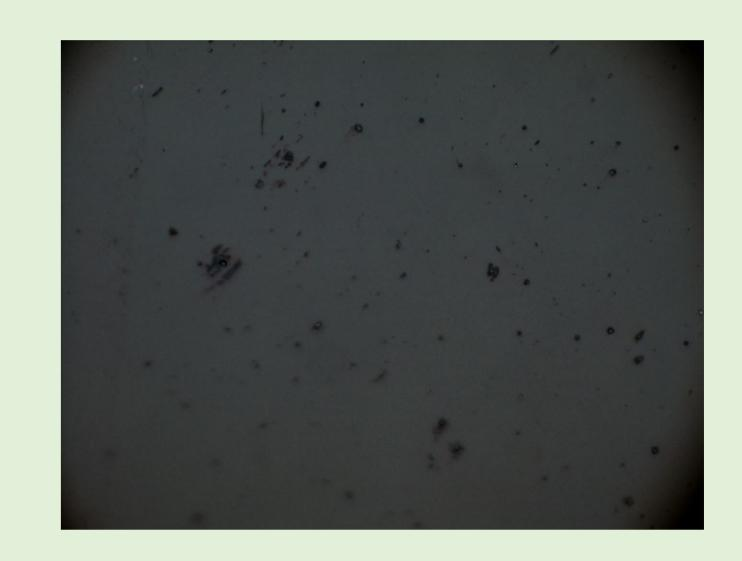
•GAXRD measurements revealed crystalline AIN films with predominant (002) orientation (i.e.,c-axis AIN) for all studied pressures. In the case of the 3 mTorr AIN film, the (002) peak shifted significantly to lower angles (high compressive stress). Similarly as for the Al<sub>2</sub>O<sub>3</sub> films, no macroparticles were observed (elimination of arcing even at long deposition runs).
