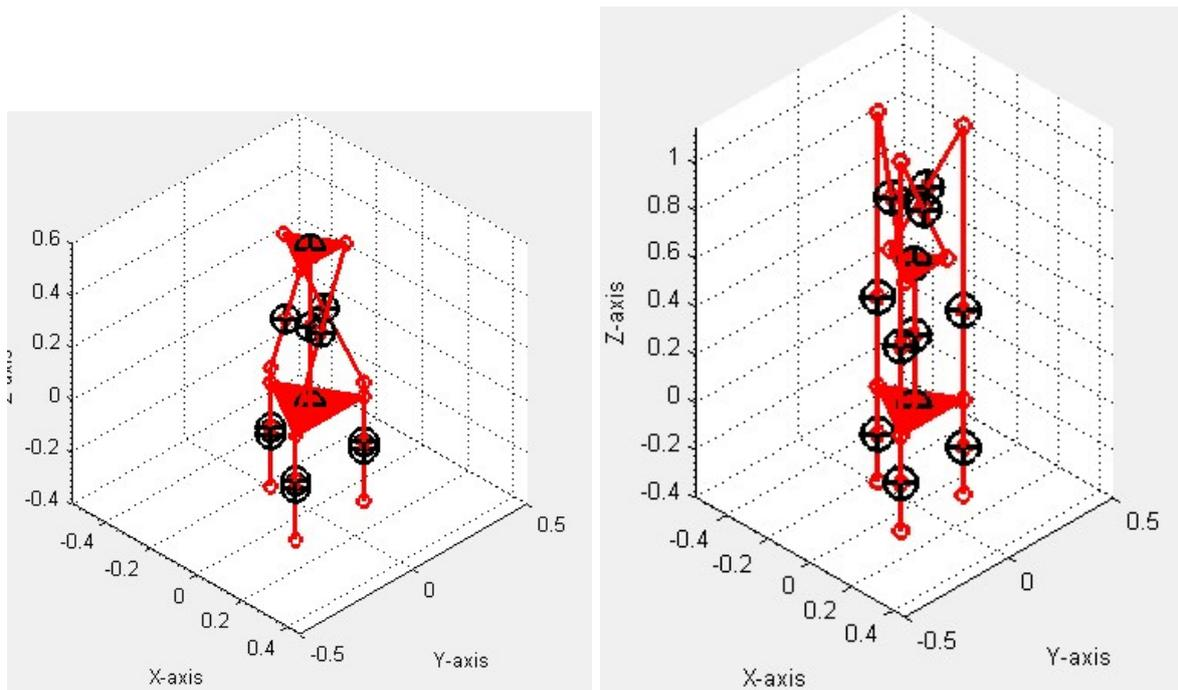
Fig. 3: Two solutions of the inverse kinematic problem of the parallel SWM
