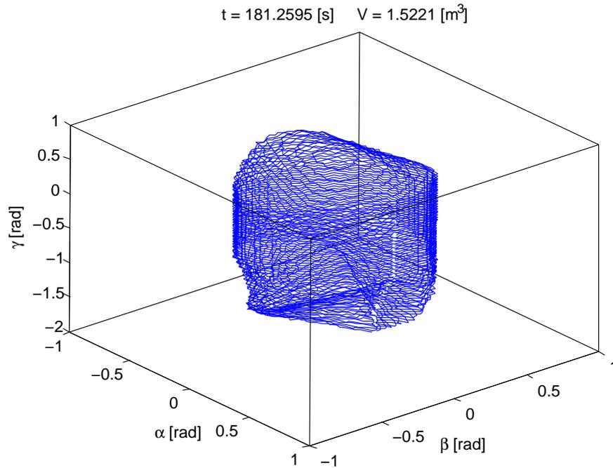
Fig. 15: Complete orientation workspace of the parallel SWM (SWBDM)
