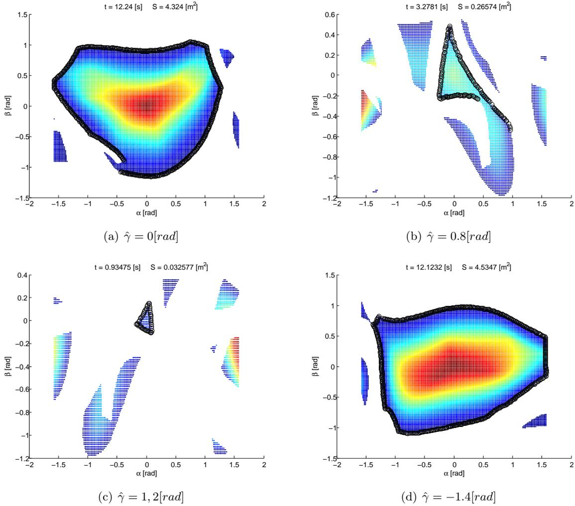
Fig. 13: Workspace of the parallel SWM (SWBDM,  $\epsilon \doteq 0.0079$ ) for the constraints  $\Delta_l^{max} = 0.5[\text{m}]$ ,  $\delta^{max} = \pi/2[\text{rad}]$ ,  $l^{min} = 0.03[\text{m}]$ ,  $\eta^{min} = 0.1$ .
