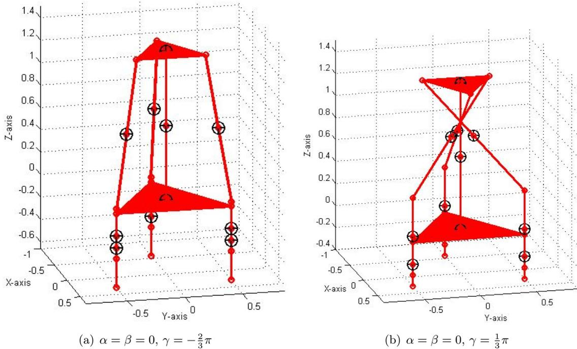
Fig. 5: Examples of the parallel singular positions of the parallel SWM
