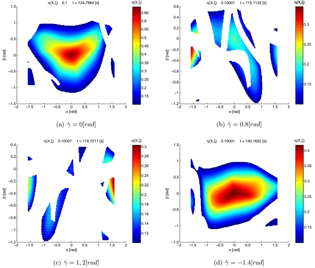
Fig. 9: Workspace of the parallel SWM (discretization method,  $N = 200 \Rightarrow \epsilon_\alpha = \epsilon_\beta \doteq 0.0158$ ) for the constraints  $\Delta_l^{max} = 0.5$  [m],  $\delta^{max} = \pi/2$  [rad],  $l^{min} = 0.03$  [m],  $\eta^{min} = 0.1$ .
