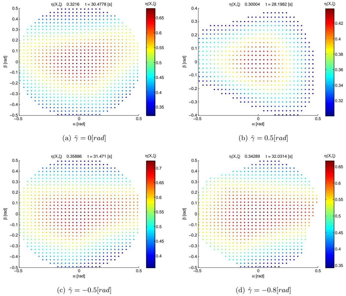
Fig. 8: Workspace of the parallel SWM (discretization method  $N = 100 \Rightarrow \epsilon_\alpha = \epsilon_\beta \doteq 0.0317$ ) for the constraints  $\Delta_l^{max} = 0.3[\text{m}]$ ,  $\delta^{max} = \pi/6[\text{rad}]$ ,  $l^{min} = 0.05[\text{m}]$ ,  $\eta^{min} = 0.3$ .
