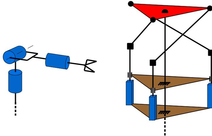
Fig. 1: The left figure: Serial SWM (Actuated revolute joints are blue.) On the right: Parallel SWM (Actuated prismatic joints are blue, black square denotes universal joint, black circle denotes spherical joint.)
