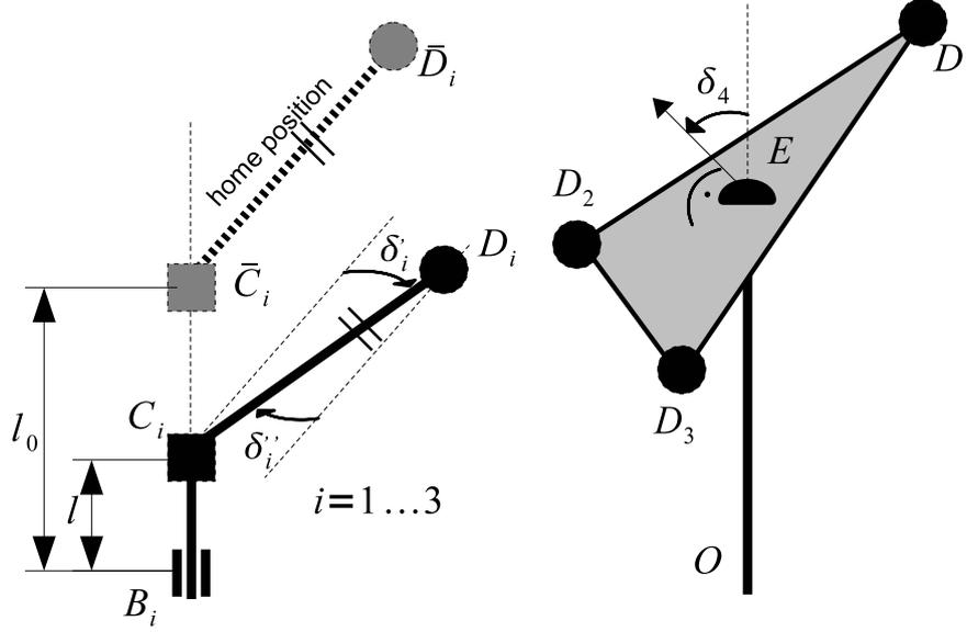
Fig. 7: Definition of the slope angles
