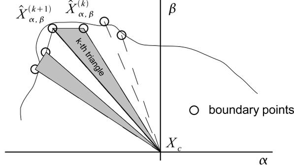
Fig. 10: Workspace boundary points and area of the layer  $\alpha\beta$ ,  $\gamma = \hat{\gamma}$
