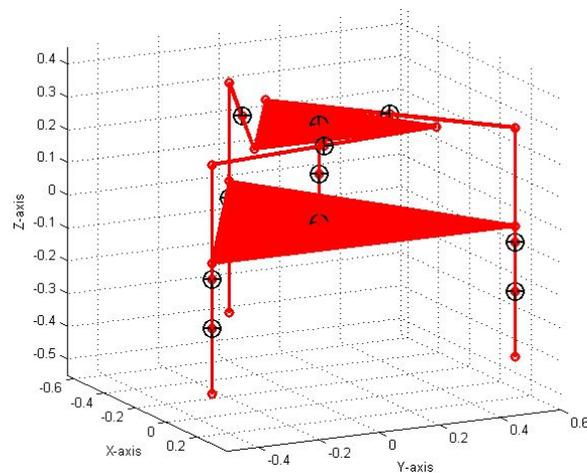
Fig. 6: Examples of the parallel and serial singular position of the parallel SWM ( $\alpha = \beta = \gamma = 0$ , the design parameters are different from the previous examples)
