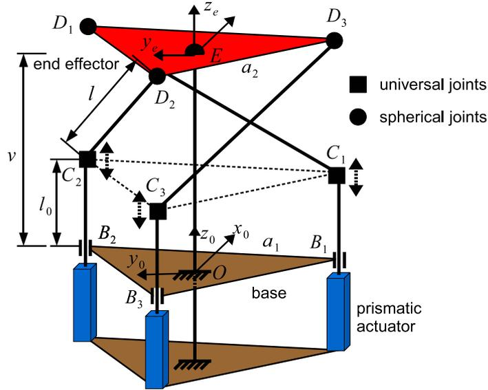
Fig. 2: Scheme of the parallel SWM in a home position
