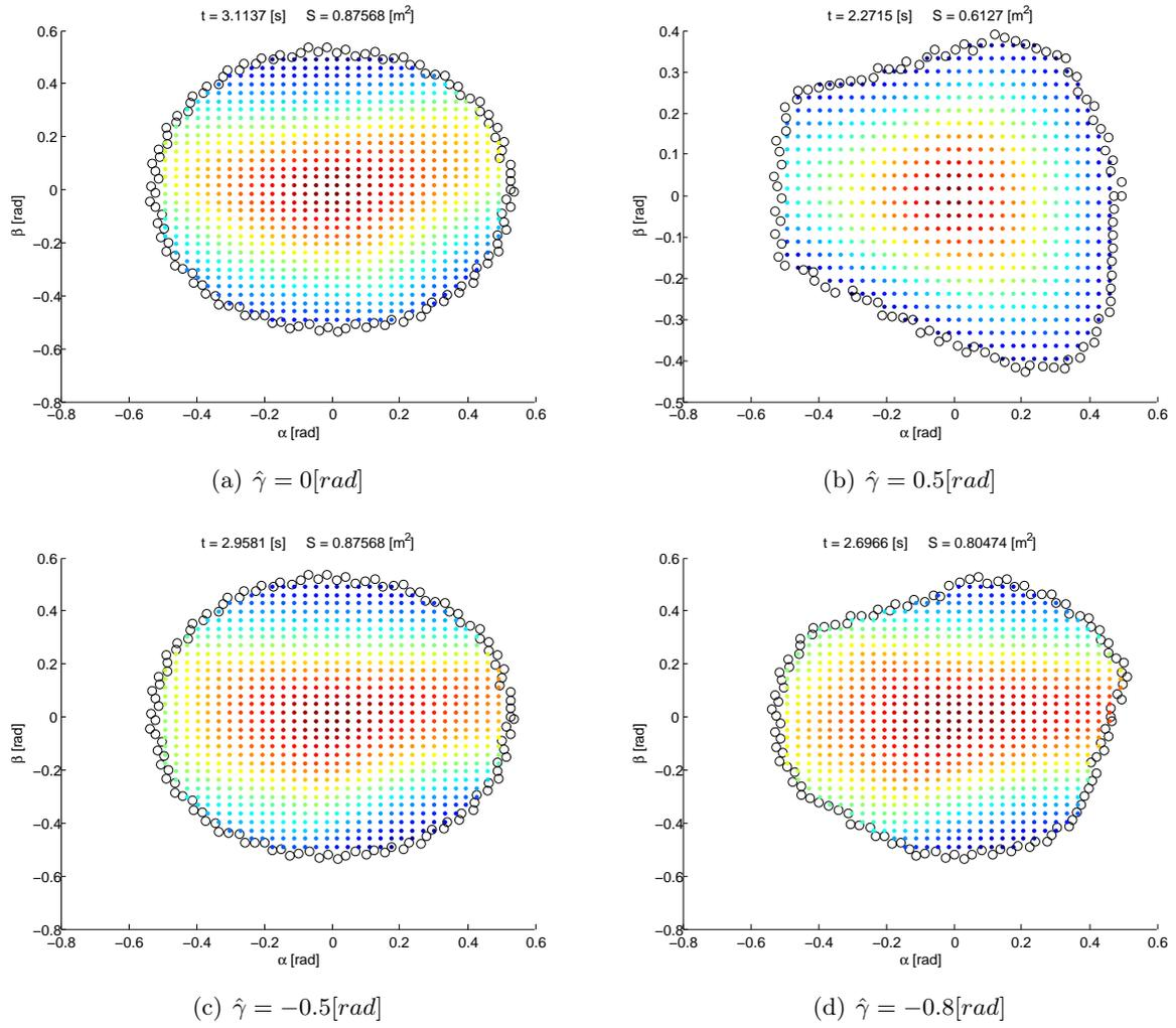
Fig. 12: Workspace of the parallel SWM (SWBDM,  $\epsilon \doteq 0.0159$ ) for the constraints  $\Delta_l^{max} = 0.3[m]$ ,  $\delta^{max} = \pi/6[\text{rad}]$ ,  $l^{min} = 0.05[m]$ ,  $\eta^{min} = 0.3$ .
