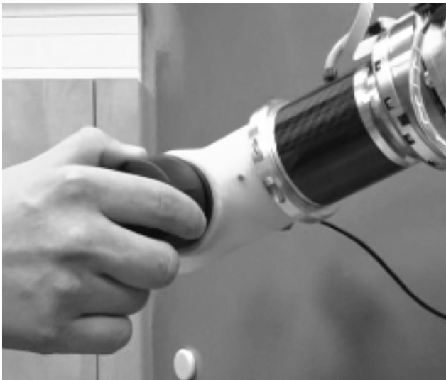
Hand guidance of the robot end-effector (left) and operator panel (right)
