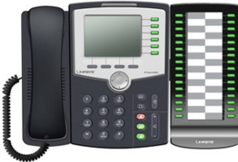
Fig. 1 – Linksys SPA962 IP phone with SPA932 extension module
