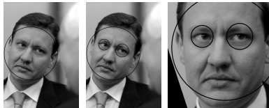
Figure 3: Example of face detection (left), eyes detection (middle) and face rotation according to the eyes (right)
