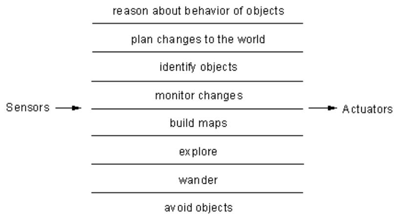
Fig. 2: Subsumption architecture (Brooks).
