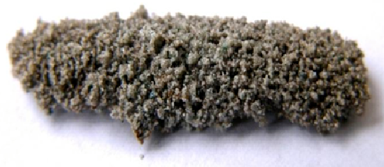
The deposit collected on the probe during combustion of agro biomass
