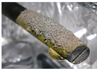
The deposit collected on the probe during combustion of agro biomass
