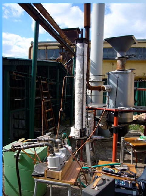
Fig. 5 Gasification device and reburning device
