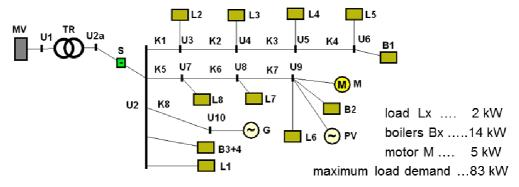
in grid-connected mode, source impedance in U6 and U9 is just equal to the EMC reference impedance
