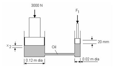
2. Calculate  $F_1$  and  $x_1$  for the case shown below.
