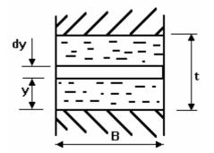
The flow through the slit is  $dQ = u Bdy = (dp/dx)(1/2\mu)\{y^2 - ty\} Bdy$ Integrating between y = 0 and y = t to find Q yields  $Q = -B(dp/dx)(t^3/12\mu)$
