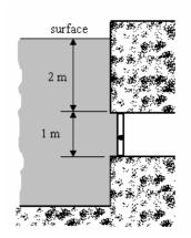
4. The diagram shows a rectangular vertical hatch breadth B and depth D. The hatch flips open when the water level outside reaches a critical depth h. Show that for this to happen the hinge must be located at a position x from the bottom given by the formula
