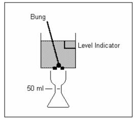
This works on the principle of allowing the fluid to run through an orifice of very accurate size in an agate block.
