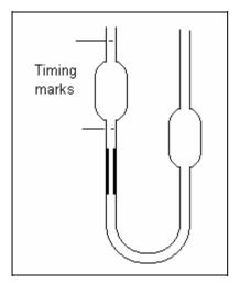
The fluid is drawn up into a reservoir and allowed to run through a capillary tube to another reservoir in the other limb of the U tube.
