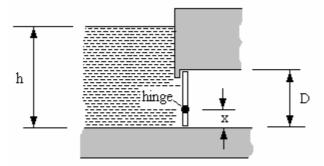
The hatch will flip open as soon as the centre of pressure rises above the hinge creating a clockwise turning moment. When the centre of pressure is below the hinge, the turning moment is anticlockwise and the hatch is prevented from turning in that direction. We must make the centre of pressure at position x.
