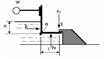
Pressure force on the bottom =  $Fp = pA = \rho gAH = 9810H$  $\overline{y} = H/2$  A = 2H  $R = \rho gA \overline{y} = \rho gAH/2 = 9810 H^2$ R acts at H/3 from the bottom Moments about O give the following.
