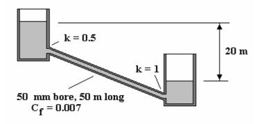
Apply Bernoulli between the free surfaces and  $h_L = 20 \text{ m}$
