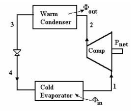
2. A vapour compression cycle uses R12. the vapour is saturated at -20°C at entry to the compressor. At exit from the compressor it is at 10.84 bar and 75°C. The condenser produces saturated liquid at 10.84 bar. The liquid is throttled, evaporated and returned to the compressor.
