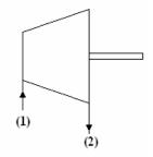
2. A gas compressor compresses gas adiabatically from 1 bar and  $15^{\circ}$ C to 10 bar with an isentropic efficiency of 0.89. The gas flow rate is 5 kg/s.
