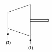
A back pressure steam cycle works as follows. The boiler produces 8 kg/s of steam at 40 bar and 500°C. This is expanded to 2 bar with an isentropic efficiency of 0.88. The pump is supplied with feed water at 0.5 bar and 30°C and delivers it to the boiler at 31°C and 40 bar.
