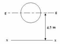
5. Find the  $2^{nd}$  moment of area for the shape shown the about the axis s – s. All the dimensions are in metres.
