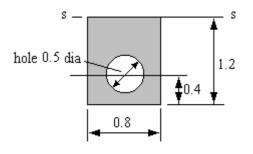
2. Find the distance of the centroid from the bottom edge. All dimensions are in metres.
