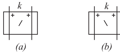
Figure 11.17: Graphical symbol for energy-transfer transformers with (a) k = n_a/n_b and (b) k = n_b/n_a .
