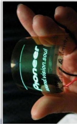
Luminescence of an organic light-emitting diode deposited onto a flexible, low CTE and optically transparent wood-cellulose nanocomposite.
