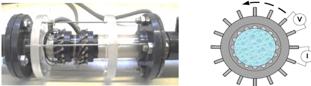
Figure 3: EIT sensor installed in 2inch pipeline
