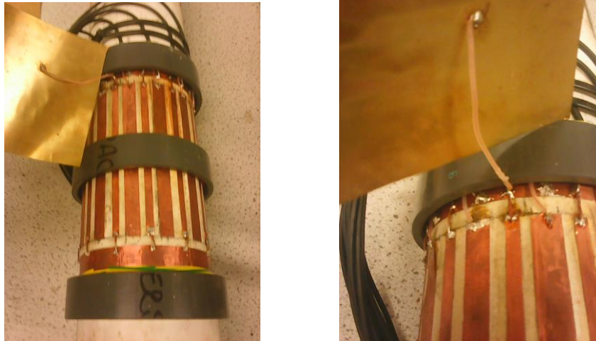
Figure 16 . View inside the ECT sensor for flame detection
