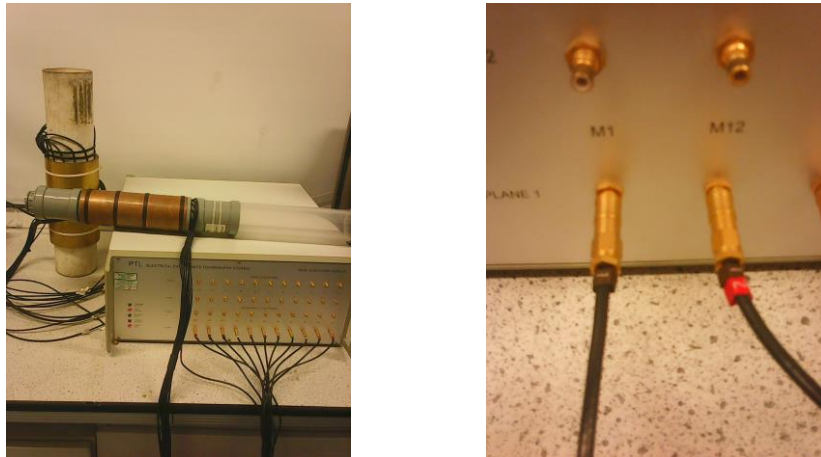
Figure 17 . Twin-plane measurement unit PTL300E from Process Tomography Ltd. and the cable connection detail
