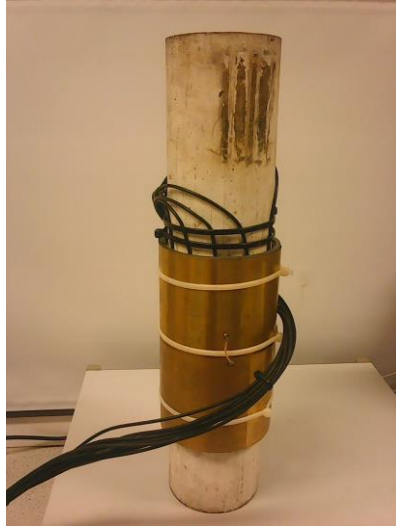
Figure 15 . ECT sensor for flame detection
