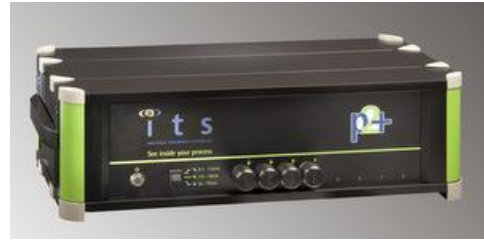
Figure 23 . EIT hardware from ITS (source http://www.itoms.com ). V5R left, P2+right
