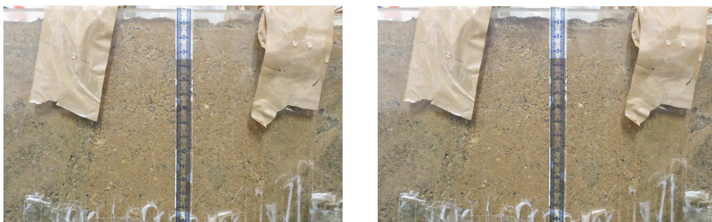
Fig. 16: Left – photograph of a tank before pouring the solution, right – after pouring the solution (only very small color change is visible at the top)
