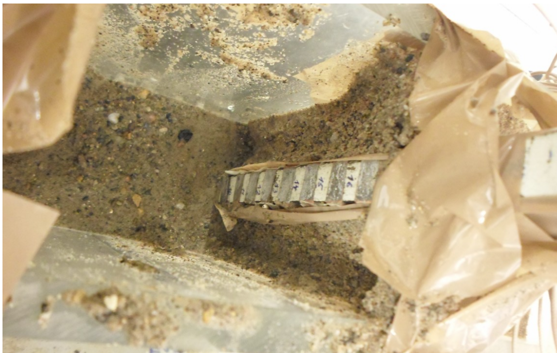
Obr. 18: Detail of soldered electrodes within the tank
